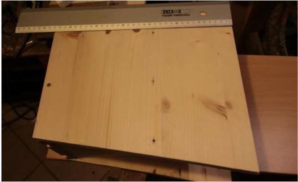
Drill three holes and attach mid wall to form the interior box for the bird nesting.
