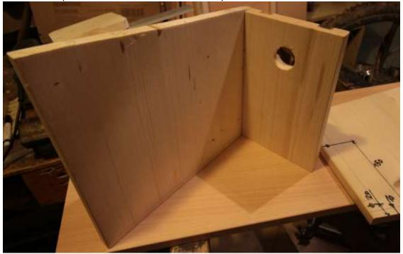
Attach both side walls and fix the floor. Warning!!! The floor must be 10mm rised.
