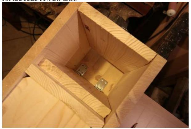
Remove the house and left the roof on the table. Try not to move the brackets (to keep the position)
