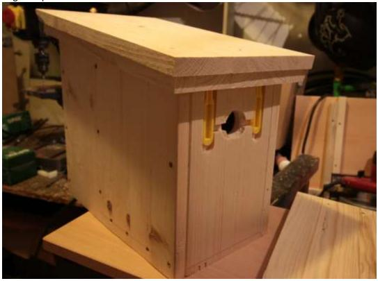
Turn upside down and mark the position. Warning: small edge must be all around the roof edge.
