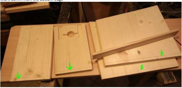
Mark position for the front on the left and right side plate (lower edge)
